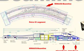
Top: Position of the Micro and Nanofocus X-ray Scattering (MINAXS) beamline within the layout of Petra III. Bottom: The nanofocus hutch is located downstream the microfocus endstation, both of which are fed by a canted undulator.
