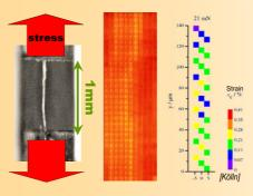
Nanofocus diffraction is complementary to TEM and SAXS/SANS as it allows for in situ experiments (e.g. temperature, mechanical load) to access single grains of polycrystalline materials on a sub-um lengthscale. Right: Microstructure of Mg-Al-Zn alloy with & w/o SiC [courtesy of GKSS].
