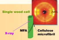
Top: Microdiffraction experiment on a wood cell with the cellulose (200) reflection being an indicator for the microfibril angle (MFA). Bottom: (left) Actual experiment, the cell is exposed to lateral stress during irradiation. Combined with a µm-sized x-ray spot the intracellular strain distribution (right) can be determined from the measured MFAdistribution (middle). Yet smaller foci allow for investigation of more finely structured materials, such as fibres, smaller cells etc.
